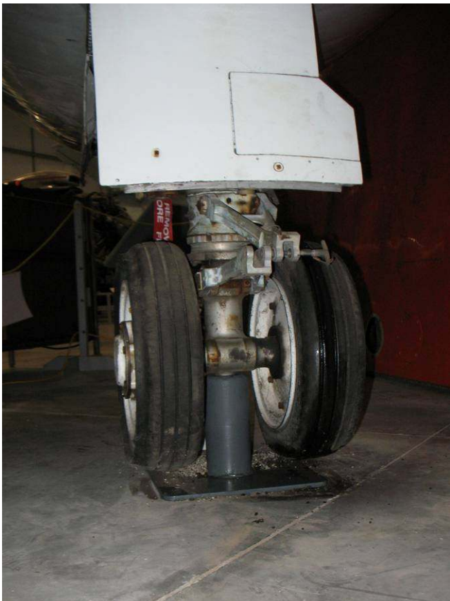
Photo – Gene Hamilton The Jetstar nose wheel with support
