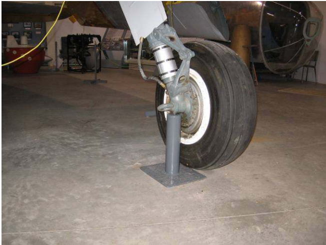
Photo – Gene Hamilton Support for the TBM
